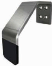
#43 Hands Free Arm Pull Surface applied, thru-bolted, 4-1/8" clearance
